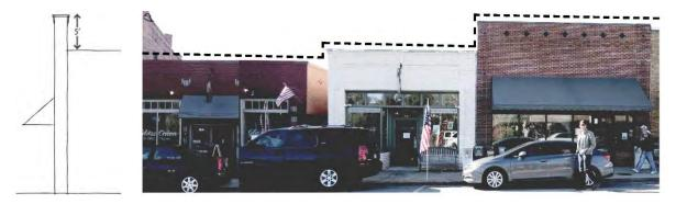
The diagrams above illustrate the maximum parapet height (left) and the relationship of adjoining parapet walls and how they come together to form a varied roof line along the block of buildings.
