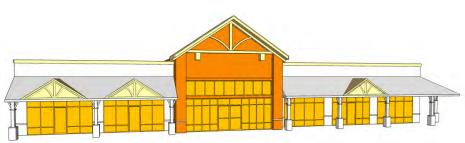
These illustrations demonstrate how individual features combine to provide vertical articulation on a building. The highlighted features include change in building height, the use of a pitched roof elements, and the use of vertical windows to achieve compliance with the vertical articulation standards.
