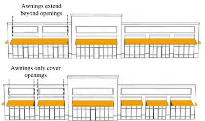
The illustrations above demonstrate the improper use (top) and proper use (bottom) of awnings. The awnings on the bottom illustration only cover the window and door openings.
