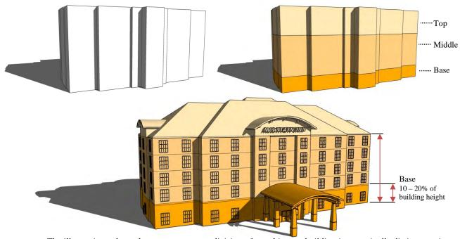
The illustrations above demonstrate proper division of a multi-story building into vertically distinct portions of the vertical wall plane, including base, body, and top sections.
