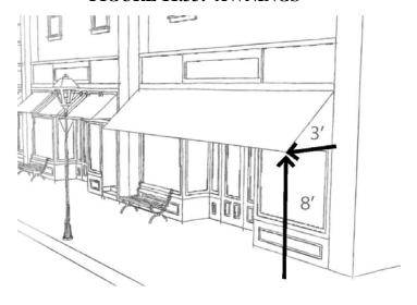
The diagram above illustrates the minimum awning depth and clearance.
